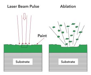
Besnovo's laser de-coating technology is an innovative alternative to the current labour-intensive, time-consuming, and environmentally-unfriendly de-coating methods such as chemical stripping, media blasting, water jet and hand sanding.
